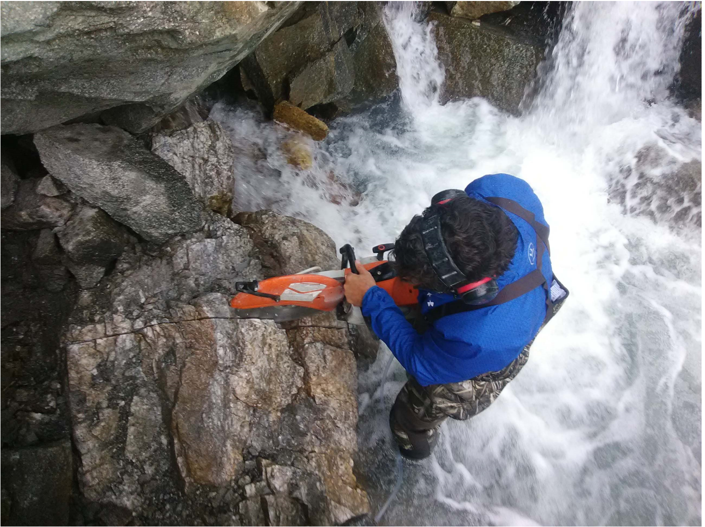
Photo 3. Crew cutting a conventional channel sample on the Goat Vein. (C. Hale, 2018).
