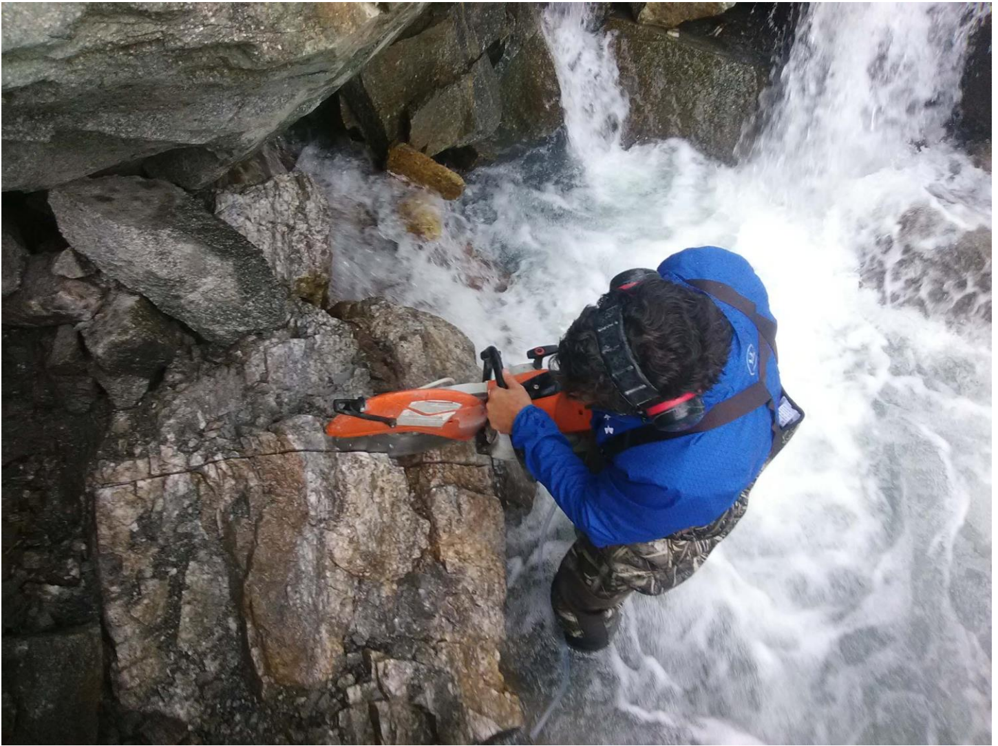
Figure 7-3: Crew cutting a conventional channel sample on the Goat Vein (C. Hale, 2018)
