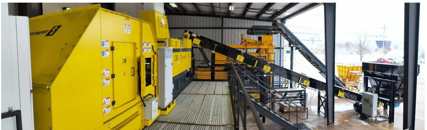
Figure 5: Steinert Sensor-Based Ore Sorting Machine
