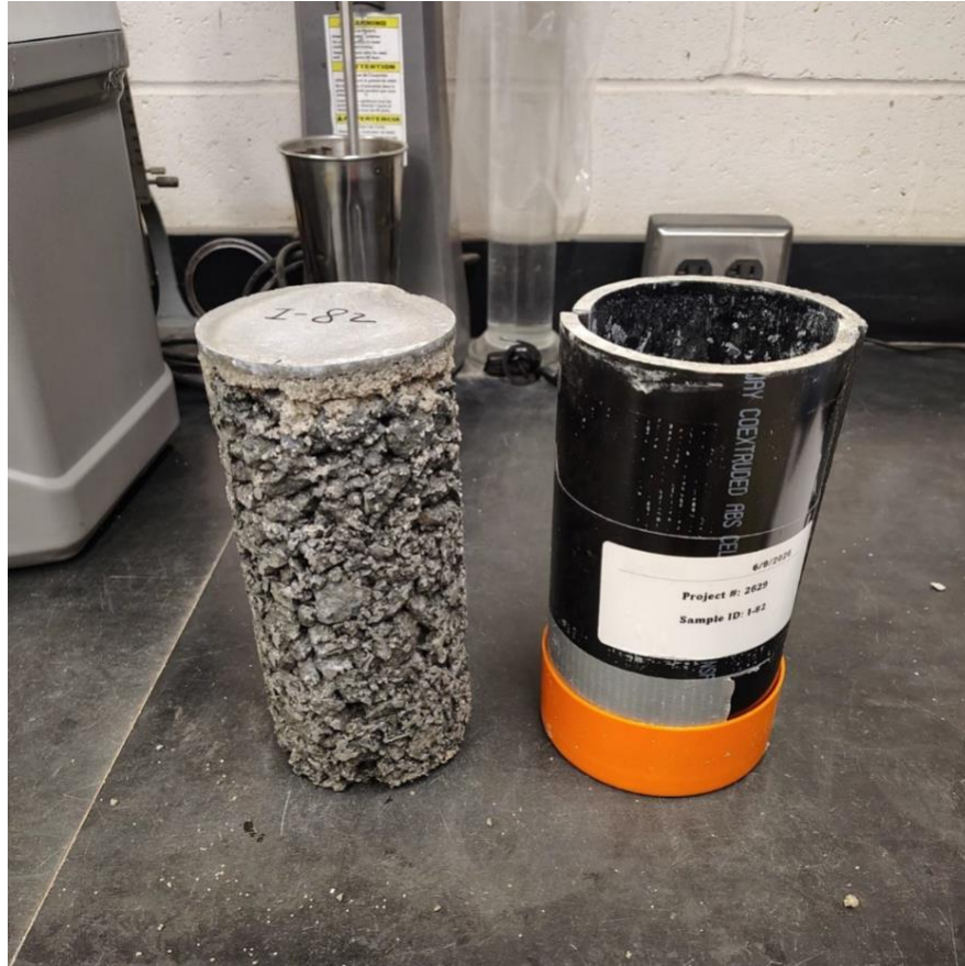
Fig. 2: Example of CRF Cylinder Cast for UCS Testing
