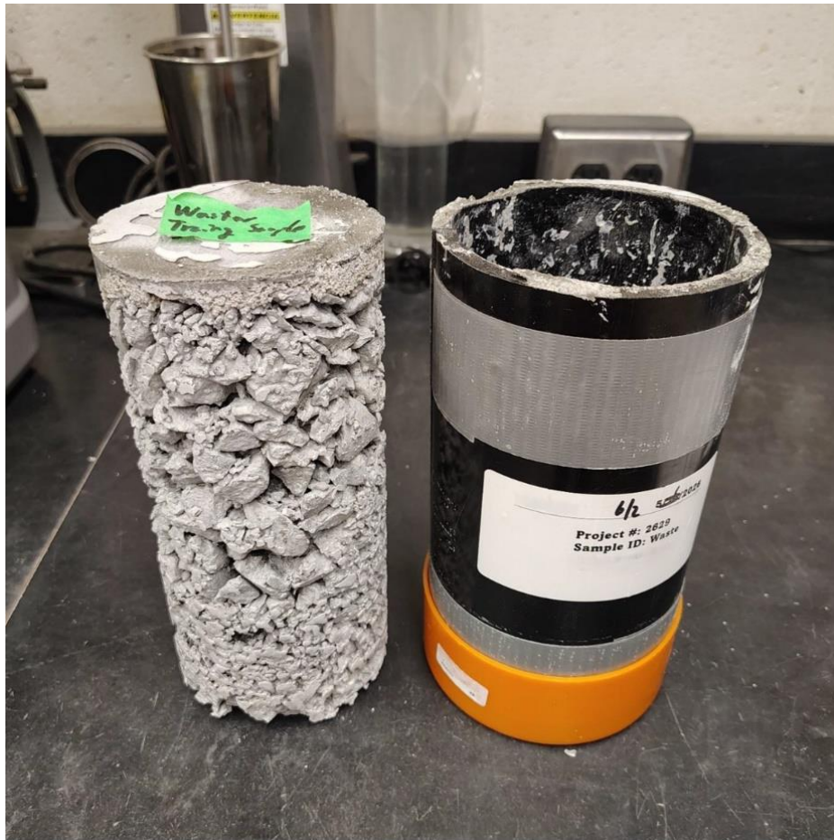
Fig. 1: Example of CRF Cylinder Cast for UCS Testing
