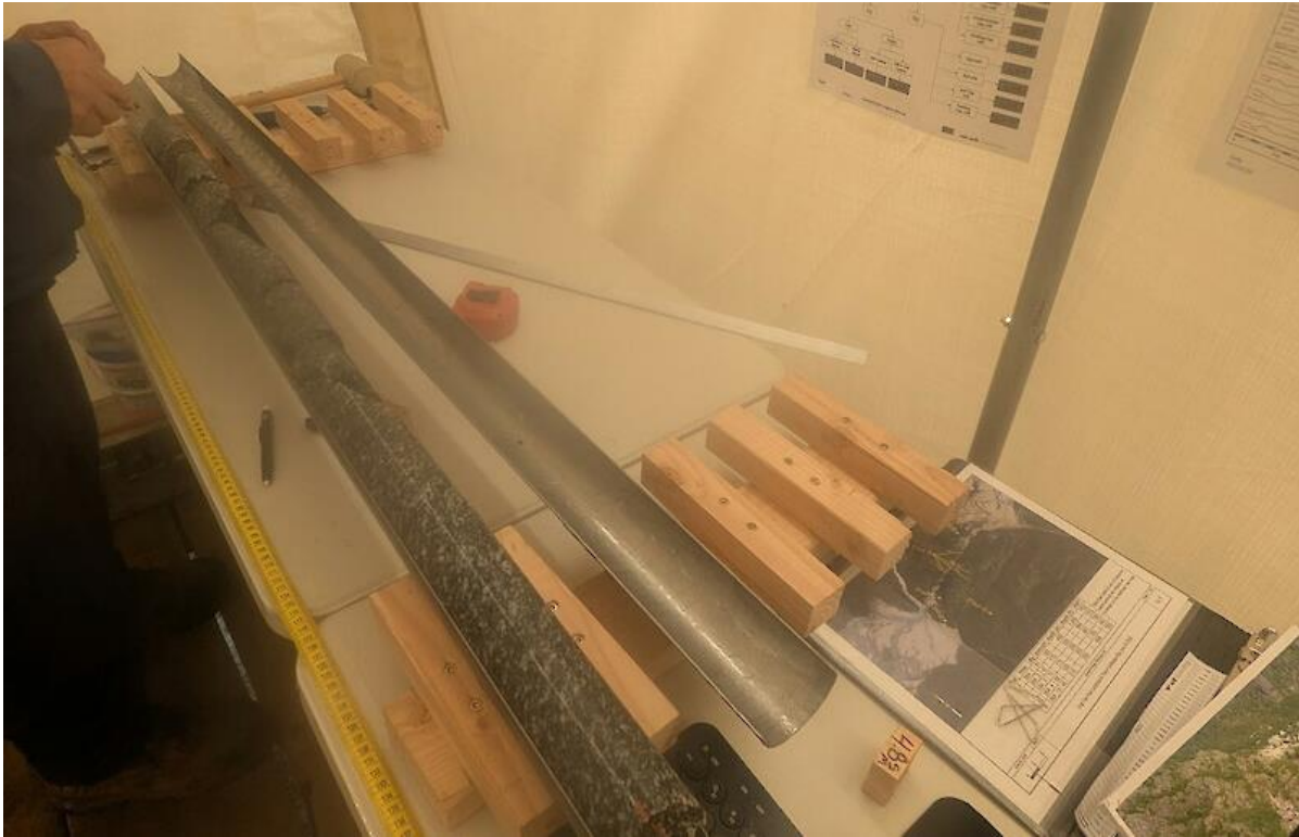
Fig. D: Logging core while still in the split-tube core barrel to preserve maximum geotechnical information
