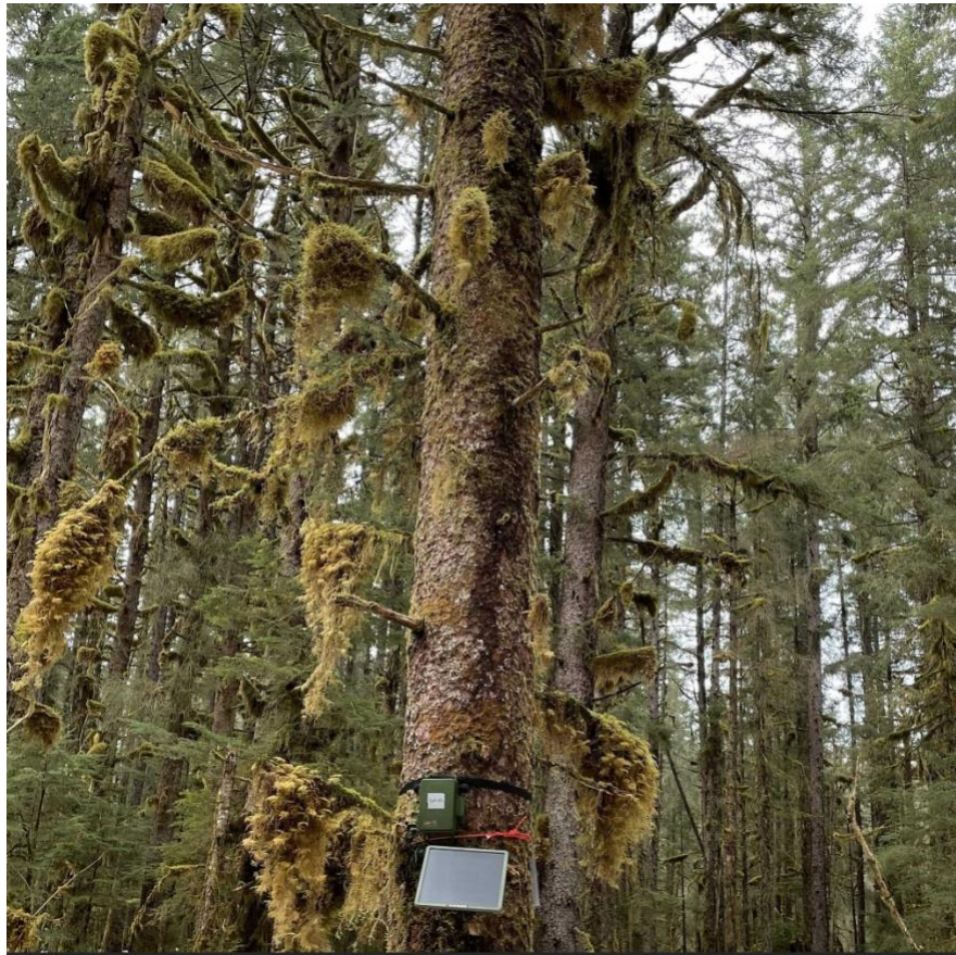
Acoustic recording unit, one of many installed in the project area to identify prevalence of relevant bird species
